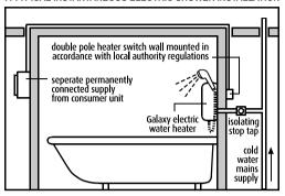
Plan your own installation carefully. Check on the nearest and most readily accessible rising mains water supply, this may be beneath the bath or in the loft, where it feeds the cold water storage tank. Use only the cold rising water main supply. Do not connect the shower unit to the down service from the tank.
