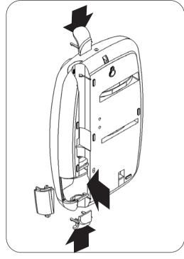
We have incorporated into the bottom right-hand side of the back plate an easy removable trim section, to allow easy access when connecting the water supply. (*Please Note!* Remember to replace this trim section before refitting the cover).
