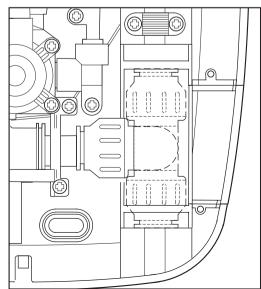
Connect the mains water supply to the inlet of the shower unit using a 15mm copper or stainless pipe. Do not use excessive force when making the connection to the unit.
